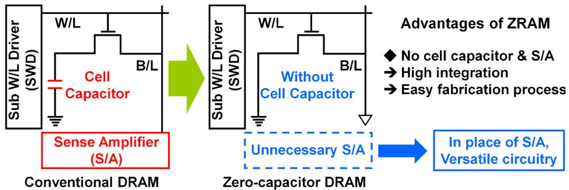
Figure 1. Comparison of conventional DRAM with 1T-1C and ZRAM with only 1T.
