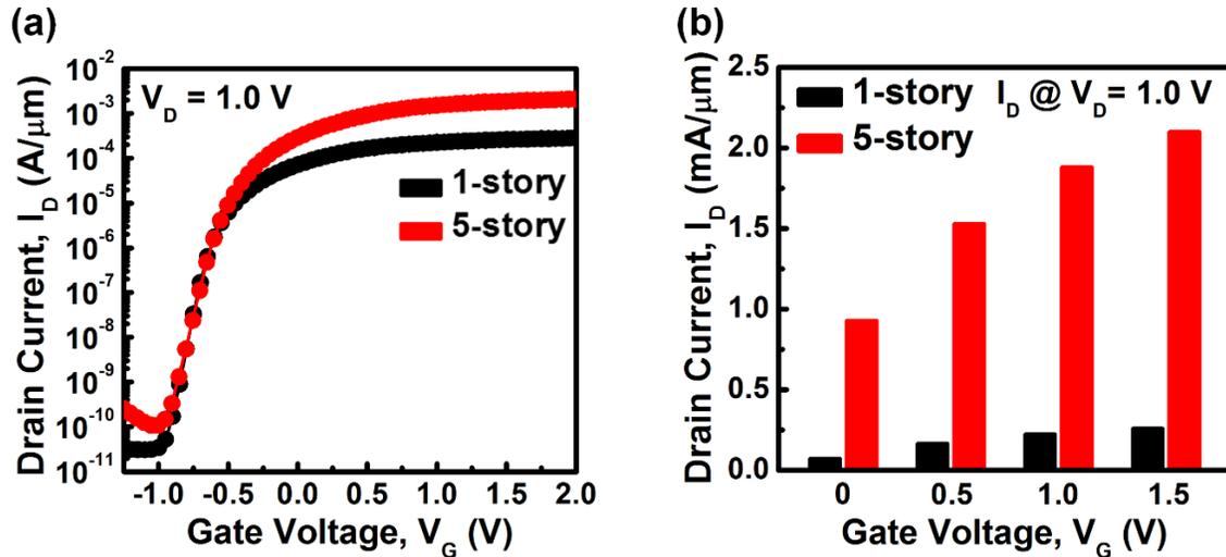
Figure 4. (a)  $I_D$ - $V_G$  characteristic of the FET with the one-story SiNW channel and the five-story SiNW channel. (b) Comparison of  $I_D$  as a function of the selected  $V_G$ .
