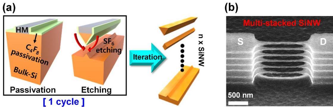
Figure 2. (a) A schematic of the ORADEP. (b) SEM image of the vertically integrated SiNW fabricated by means of the ORADEP.
