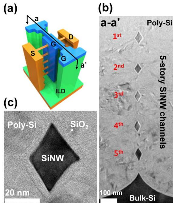
Figure 3. (a) A schematic of the fabricated device. (b) TEM image of the fabricated device. (c) Enlarged image of the SiNW in Figure 3(b).
