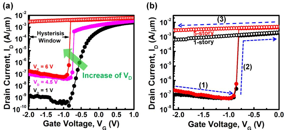
Figure 5. (a) ZRAM operation with a hysteresis loop during positive and negative bias sweeps. (b) Comparison of the ZRAM operation between ZRAM with a one-story SiNW channel and that with a five-story SiNW channel. Compared to the one-story SiNW ZRAM, an increased sensing memory window is identified in the five-story SiNW ZRAM.
