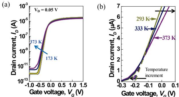
Fig. 3. (a) Transfer curve in a temperature range of 173 K to 373 K, and (b) close-up view of (a) converted to a linear-linear plot
