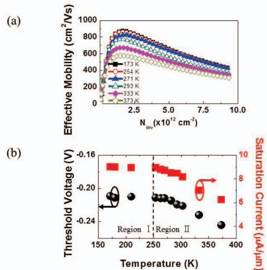
Fig. 4. (a) Temperature dependence of the effective mobility, and (b) temperature dependence of the threshold voltage and the saturated drain current. The threshold voltage was determined from the x-intercept point, which was projected from the linearly extrapolated line on the maximum  $g_m$  point. The saturated drain current was read at gate and drain voltage of 1.0 V
