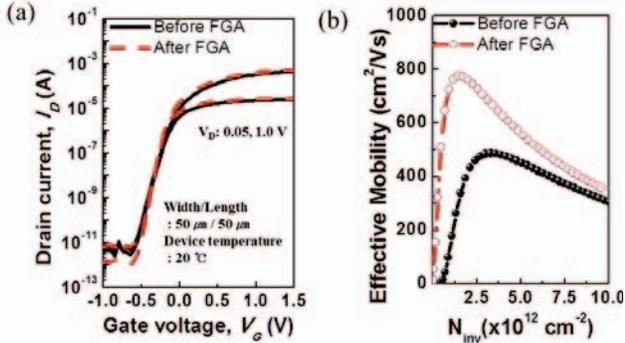
Fig. 2. Comparison of (a) the transfer curve and (b) the effective mobility before and after the FGA process. The effective mobility was extracted from measured data by the split C-V method
