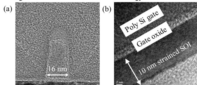
Fig. 1. High-resolution cross-sectional TEM images. (a) 16-nm gate length, (b) 10-nm channel thickness
