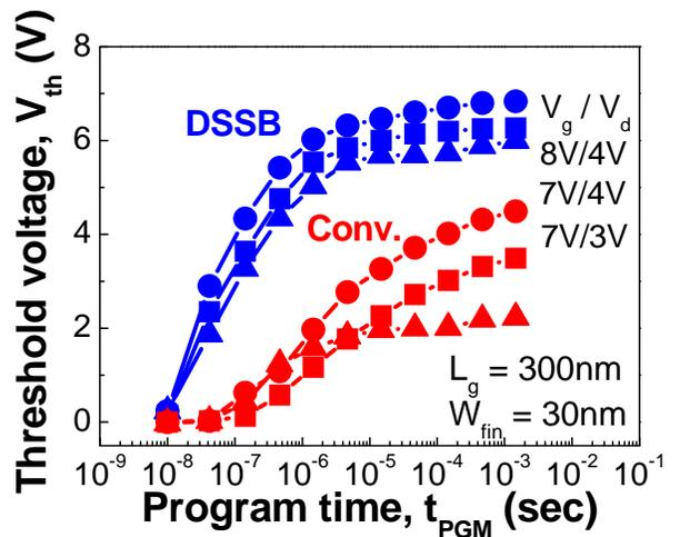
Fig. 5. Comparison of programming characteristics between conventional and DSSB FinFET SONOS.
