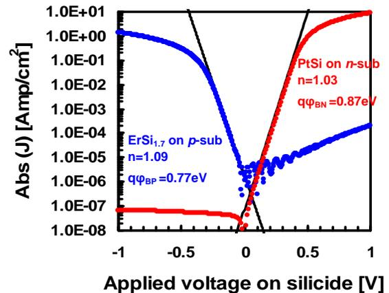
Fig. 1. Schottky diode I-V characteristics
