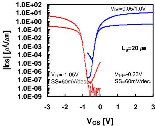
Fig. 2.  $I_{DS}$ - $V_{GS}$  characteristics of  $20\mu\text{m}$   $n/p$ -type SB-MOSFET.
