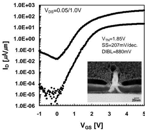
Fig. 3.  $I_{DS}$ - $V_{GS}$  characteristics of 7 nm n-type SB-MOSFET.
