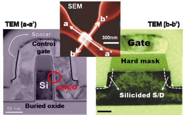
Fig. 4. Fabricated DSSB FinFET SONOS
