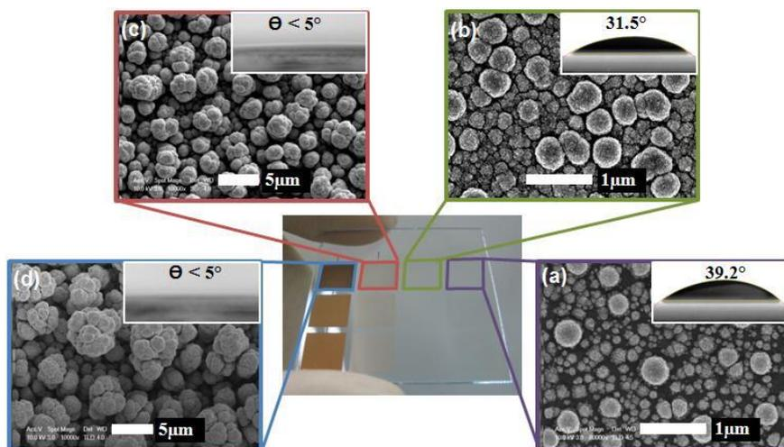
Figure 1:  $\text{HAuCl}_4$  modified  $3 \times 4$  ITO pattern array on a glass substrate (center). SEM images and corresponding contact angle measurements of the patterns after an electrochemical deposition time of (a) 1 minute, (b) 5 minutes, (c) 1 hour, and (d) 2 hours.
