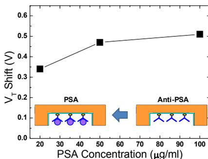
Figure 6: Dependency of the  $V_T$  shift on the PSA concentration
