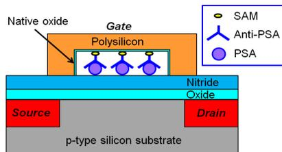
Figure 1: A cross-sectional view of the proposed FET with a vertical nanogap. The nanogap is filled with PSA and anti-PSA, causing a shift of the threshold voltage.
