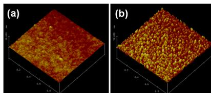
Figure 5: AFM images (a) before the chemical treatment and (b) after PSA binding on a silicon dioxide surface
