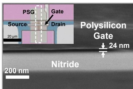
Figure 3: Images of the fabricated device. The inset shows the top view of the device taken with an optical microscope. The dotted line indicates the PSG sacrificial layer. The background SEM image shows that the vertical nanogap is properly formed.
