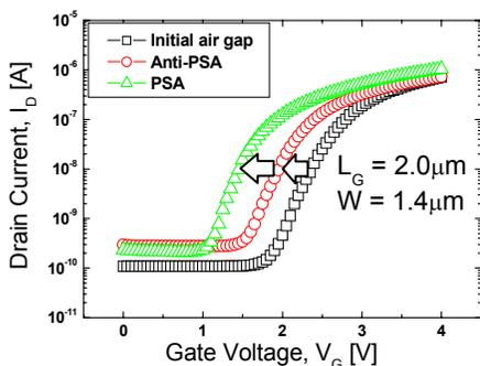
Figure 4: Transfer characteristics ( $I_D$ - $V_G$  curves) measured by a semiconductor parameter analyzer (HP4156C). 50mV was applied to the drain. The concentration of Anti-PSA and PSA was 100 $\mu$ g/ml.
