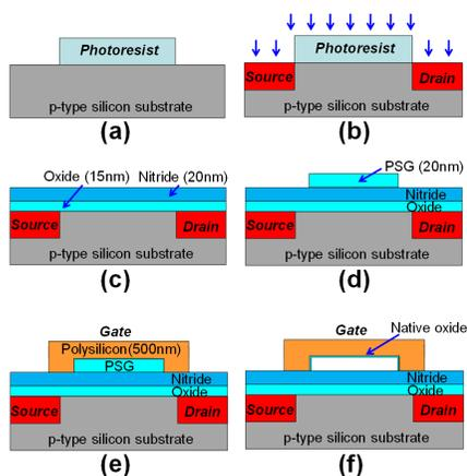
Figure 2: The process flow. (a) Photoresist is coated. (b) A source/drain junction is formed on a p-type silicon substrate by ion implantation. (c) A thermal oxide (15nm) is grown and a nitride (20nm) is sequentially deposited. (d) A 20nm thick phosphosilicate glass (PSG) sacrificial layer is deposited and patterned. (e) N+ in-situ doped polysilicon (500nm) is deposited and delineated. (f) The PSG sacrificial layer is removed by buffered oxide etchant.
