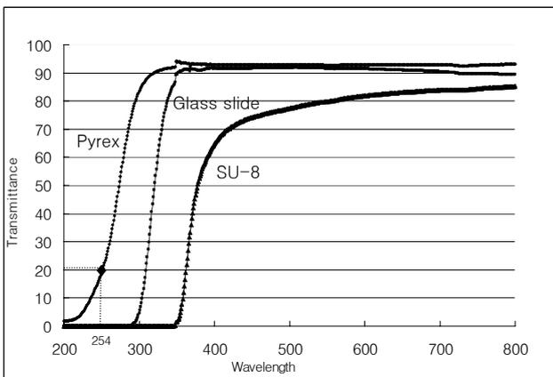
Figure 3. Transmittance (%) values for Pyrex, glass slide, and SU-8 (100µm)
