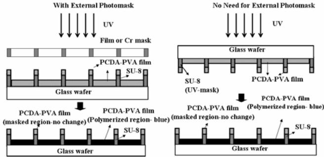
Figure 2. Comparison of the composite-polymer patterning methods with external and chip embedded SU-8 mask
