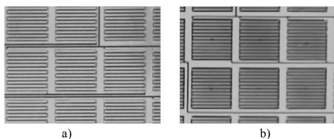
Figure 5. 30µm SU-8 and micro-heater structure a) before and b) after 254nm UV irradiation for 10 minutes
