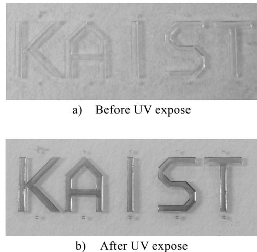
Figure 4. PCDA+PVA composite film layer on SU-8
