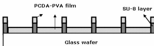
Figure 1. Structure of the chip embedded SU-8 photomask
