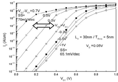
Fig. 7. Electrical characteristic at the synchronized mode operation with various bias effects. ( $V_{G1}$  and  $V_{G2}$  start from the same or the different initial biases and varies simultaneously).
