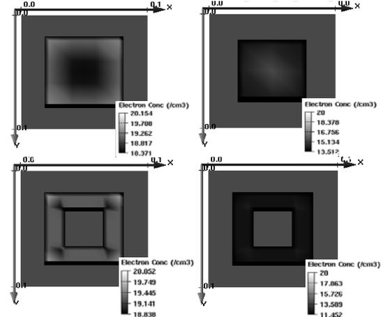
(a) Nano-wire at  $V_G = 1V / V_D = 1V$  (b) Nano-wire at  $V_G = 0.3V / V_D = 1V$
