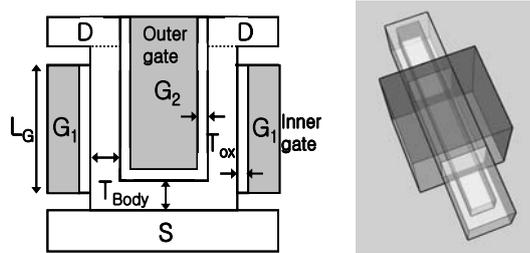
Fig. 2. Schematic of the simulated vertical nano-shell AAG MOSFET.
