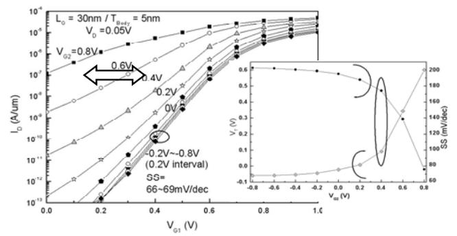
Fig. 8. Electrical characteristic at the static mode ( $V_{G1}$  varies with fixed  $V_{G2}$  bias). The inset shows  $V_T$  and S.S. as a function of  $V_{G2}$ .
