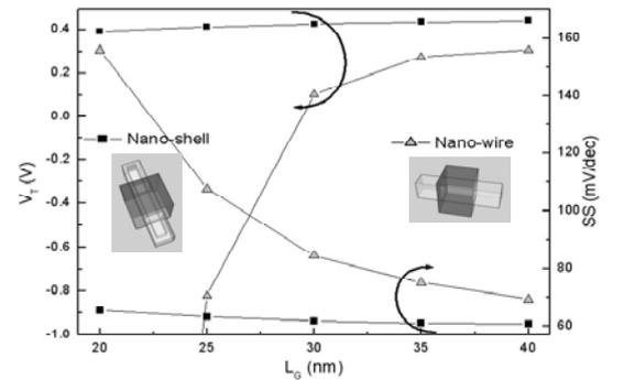
Fig. 4.  $V_T$  roll-off and S.S. versus  $L_G$  in the nano-wire (Single AAG) and nano-shell FET (Double AAG).
