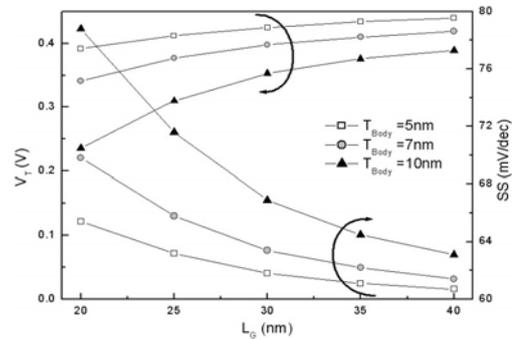
Fig. 6. Body thickness modulation effect on  $V_T$ -roll off and S.S.
