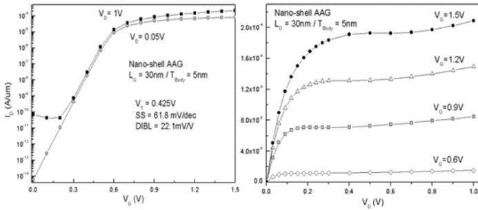
Fig. 3.  $I_D$ - $V_G$  and  $I_D$ - $V_D$  characteristics of the vertical nano-shell AAG MOSFET (at the synchronized mode operation).
