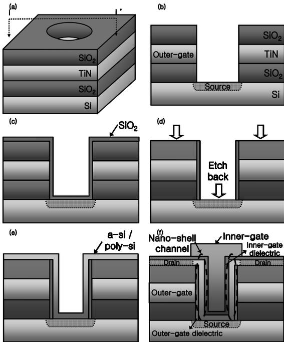
Fig. 1. Process flow of the vertical nano-shell AAG MOSFET.
