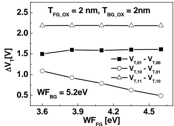
Fig.3. A shift of threshold voltage characteristics for various front gate workfunctions.
