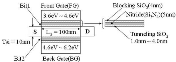
Fig.1. Schematics of ASDG NVM cell
