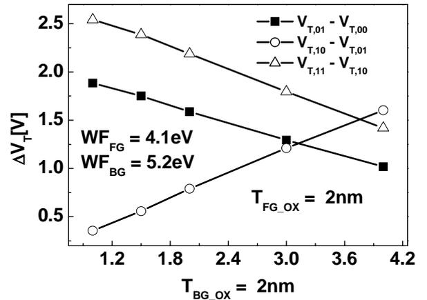
Fig.6. The shift of threshold voltage characteristics for various front gate oxide thickness.
