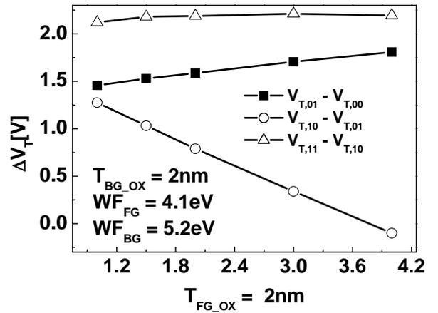
Fig.5. The shift of threshold voltage characteristics for various back gate oxide thickness.
