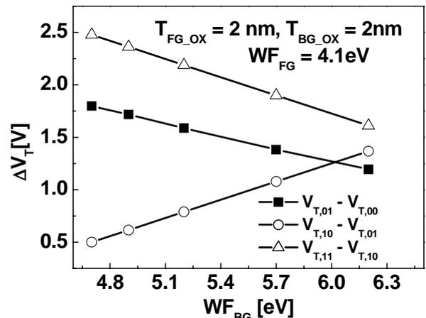
Fig.4. A shift of threshold voltage characteristics for various back gate workfunctions.
