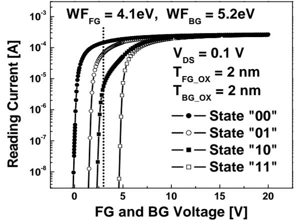
Fig.2. I-V characteristics of the ASDG cell programmed with the 4 distinguishable states of “00”, “01”, “10”, and “11”.
