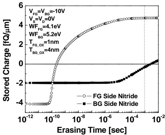
Fig.8. Transient behaviors of the stored charges at the interfacial nitride of FG and BG side during erase operation.
