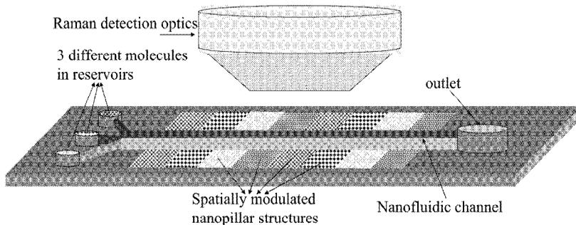
**Figure 1.** Conceptual schematics of multiplexed SERS detection of biomolecules transported in nanofluidic channel. The SERS substrate above is spatially modulated with variant surface densities of nanopillars and optimized for different molecules.
