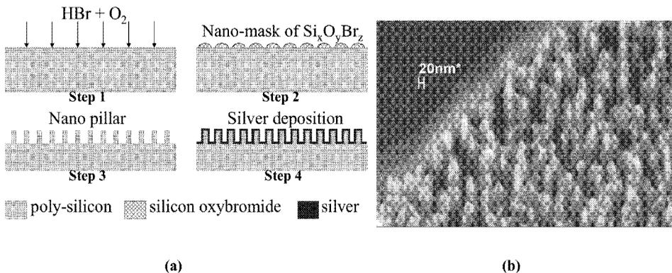
**Figure 2.** (a) Fabrication process of nanopillar SERS substrate. (b) SEM image of NanoHARP shows high-aspect-ratio pillars formed at polysilicon surface arranged in statistical orders.
