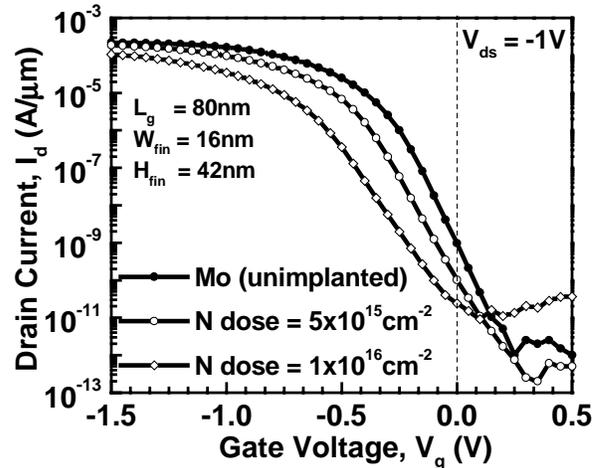
**Figure 4:**  $I_D$ - $V_G$  characteristics of Mo-gated FinFETs. Nitrogen implantation into the Mo gate can controllably alter the device  $V_T$ .
