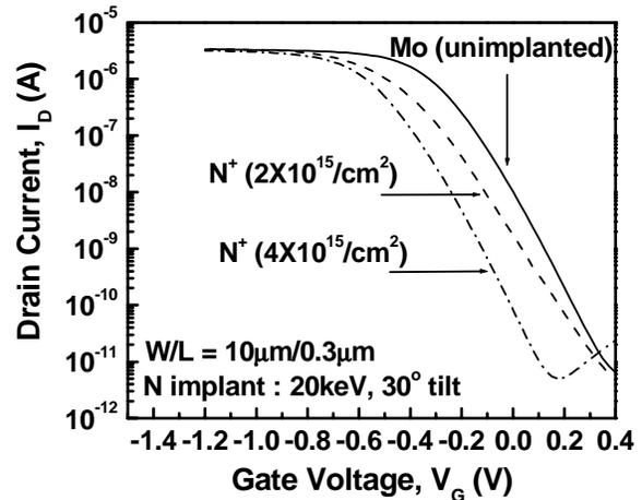
**Figure 2:**  $I_D$ - $V_G$  characteristics of Mo-gated UTBFETs. The effect of N implantation on  $V_T$  is clearly seen.
