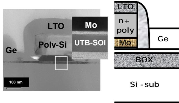
**Figure 1:** Schematic cross-section of Mo-gated UTBFET and corresponding high-resolution TEM of an actual device.
