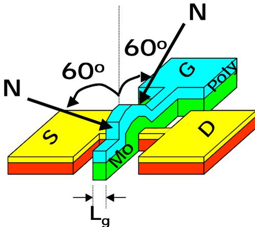
**Figure 3:** Schematic view of a FinFET with the poly-Si/Mo gate stack used. N implantation was performed twice to introduce N into both the front and back gates.
