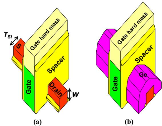
**Figure 10:** Illustration of raised-S/D fabrication process for a FinFET. (a) Structure after formation of gate-sidewall spacers. (The hardmask on top of the fin in the S/D contact regions is removed during the spacer etch.) (b) Structure after selective germanium deposition.
