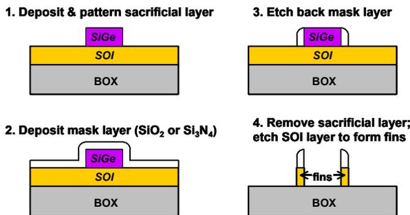
**Figure 8:** Sequence of schematic cross-sections illustrating the process for forming sub-lithographic fins using sidewall spacers as a hard mask.
