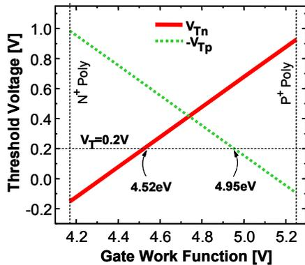
**Figure 3:** Dependence of n-channel threshold voltage (V<sub>Tn</sub>) and p-channel threshold voltage (V<sub>Tp</sub>) on gate work function, for fully-depleted SOI MOSFETs [11].
