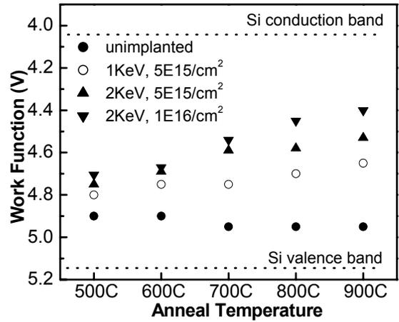
**Figure 5:** Dependence of Mo gate work function on post-N<sup>+</sup>-implant annealing temperature and implant parameters [16]. All anneals were 15 minutes long, except for the 900°C anneal (15 seconds).
