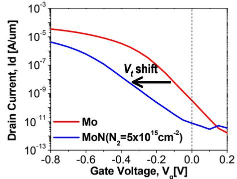
**Figure 6:** Measured transfer characteristics (I<sub>D</sub> vs. V<sub>G</sub>) of Mo-gated p-channel FinFETs (L<sub>g</sub>=80nm, W<sub>fin</sub>=10nm). Note that |V<sub>T</sub>|=0.2V (defined at I<sub>D</sub>=100nA/μm) is achieved without heavy body doping. Nitrogen implantation is effective for adjusting V<sub>T</sub>.
