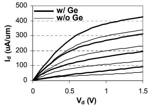
**Figure 11:** Measured output characteristics (I<sub>D</sub> vs. V<sub>D</sub>) of n-channel FinFETs with L<sub>g</sub>=90nm and W<sub>fin</sub>=70nm [22]. Significant improvement in drive current is achieved with the raised Ge-S/D structure.
