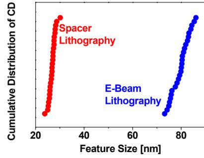
**Figure 9:** Comparison of CD uniformity achieved with a sidewall-spacer hard-mask process against that achieved with an e-beam lithography process [19].
