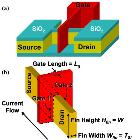
**Figure 1:** (a) Quasi-planar FinFET structure. A SiO<sub>2</sub> hard mask is used to protect the top of the SOI film during the long gate-etch process. (b) Key structural parameters are labelled. (Note that the oxide hard mask is not shown in this illustration for simplicity.)
