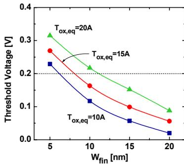
**Figure 2:** Dependence of FinFET threshold voltage on fin width and gate-oxide thickness for asymmetric (n<sup>+</sup>/p<sup>+</sup> poly-Si) gates [9].
