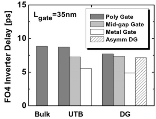
**Figure 4:** Comparison of loaded-inverter delay for thin-body SOI CMOS technologies against that for bulk-Si CMOS technology.
