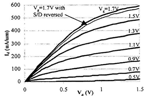
Fig. 7.  $I_d-V_d$  for FinFET with poor misalignment. The thinner line for  $V_g = 1.7\text{V}$  shows the effect of reversing the source and drain connections.
