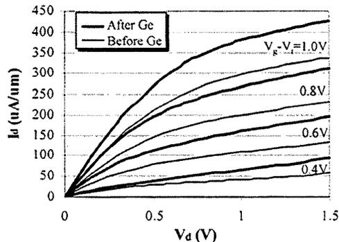
Fig. 6.  $I_d-V_d$  for  $L_g/W_{fin} = 90/70\text{nm}$  single fin FinFET. A 28% increase in  $I_{dsat}$  results from Ge raised S/D.  $W = 2 * (\text{fin height}) = 100\text{nm}$ .
