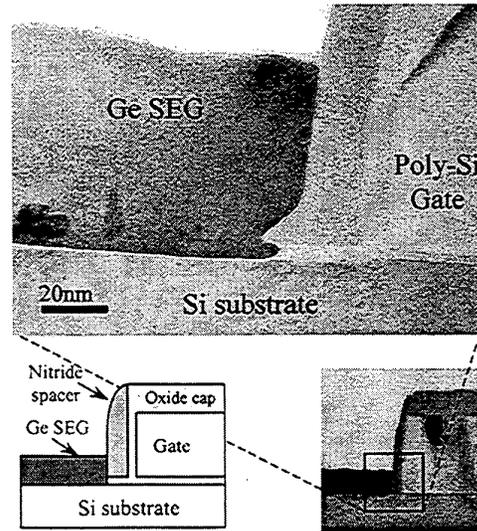
Fig. 4. TEM cross-sectional image of selectively grown Ge on a bulk-Si test wafer. The deposition is perfectly selective to both nitride and oxide.
