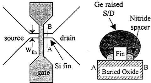
Fig. 2. FinFET layout and cross sectional view. The cross section shows the fin after selective growth of ~70nm raised S/D.
