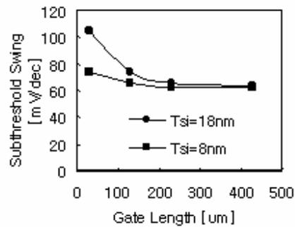
Fig. 6 Subthreshold swing dependence on gate length ( $L_g$ ) and body thickness ( $T_{si}$ ).
