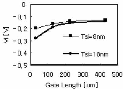
Fig. 5 Threshold voltage dependence on gate length ( $L_g$ ) and body thickness ( $T_{si}$ ).
