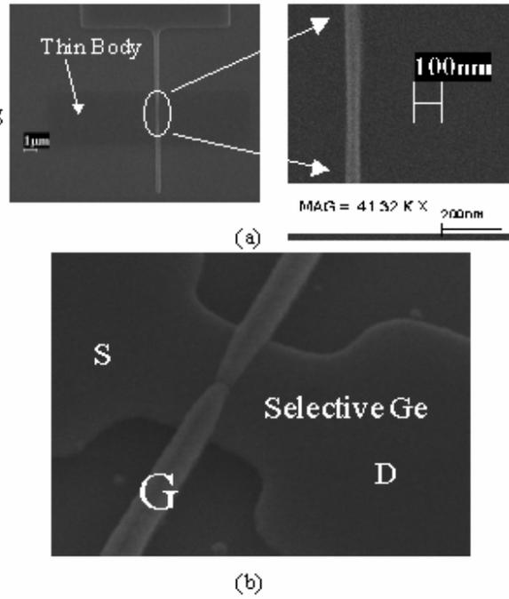
Fig. 2 SEM pictures of (a) 30nm gate length and (b) selectively deposited Ge raised S/D.
